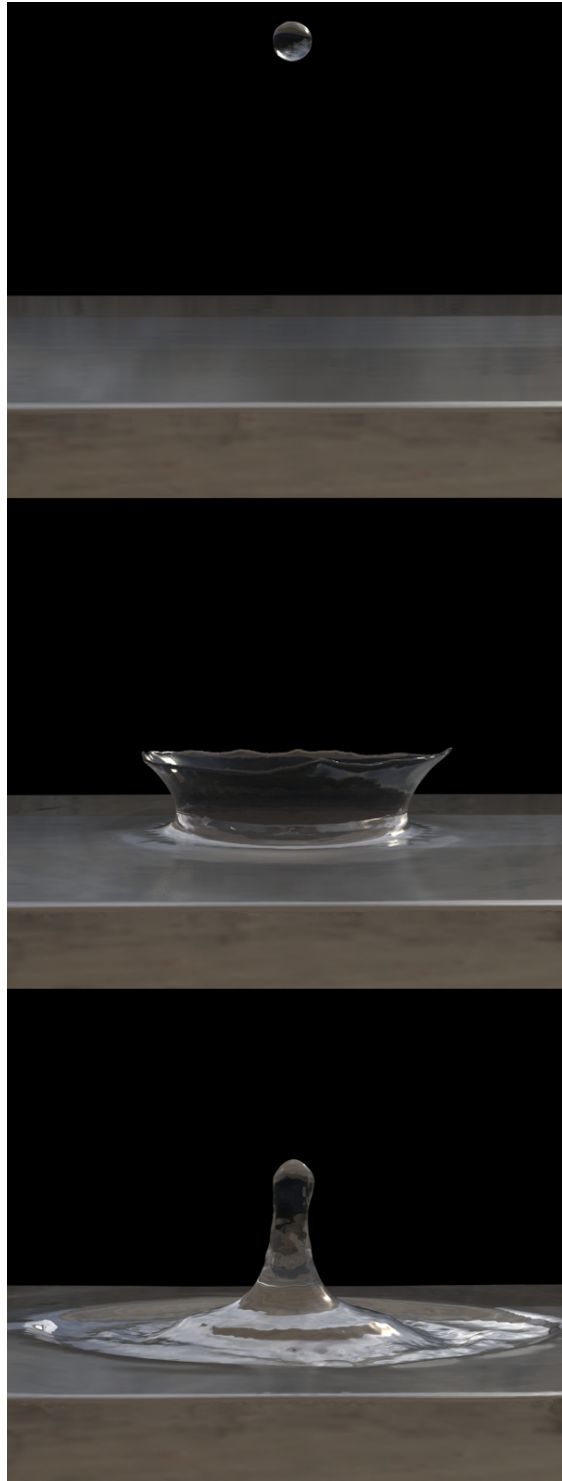
Figure 5.2: An example of a crown splash simulated using our linear octree structure. Notice that the fine details occur at the fluid surface while there is very little going on below the surface.
